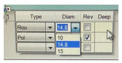
• Make sure that each hole or figure is made with the appropriate tool. To do this, click on each figure and select the appropriate auger for the thickness of the glass. The number of the auger or router is defined by the operator, for example, in the photo, the 10 is a 3/8 router, the
