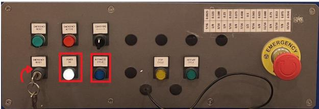
First, turn the key to reset the alarms, then press the Power on button, and finally select Automatic Cycle.
