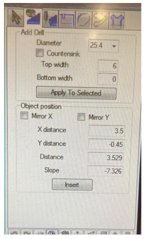
• To add holes to a drawing, you must select the second tab from the top right and define the diameter of the hole, then move the cursor over the drawing and the hole will be displayed, simply click on the final position of the hole.
