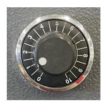
With this wheel you will control speed which the glass passes through the polisher, ideally the speed for each type of glass should be the following:
