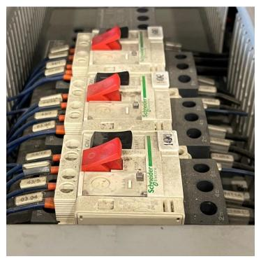
**Motor alarm:** In case a motor alarm shows up on the screen, the machine must be opened and check if any of the switches have tripped, all the brakes must have the red part up and the black part down.
