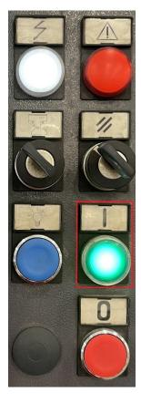
3. To finish the machine initialization, press the flashing green button.
