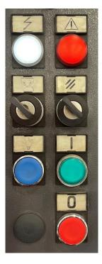
2.2 Press the green button under the key you rotated previously, it should turn on.
