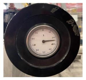
With this wheel the height of the glass to the polishing wheel is controlled, the higher the number, the lower the height will be, and the stones will scabble more.
