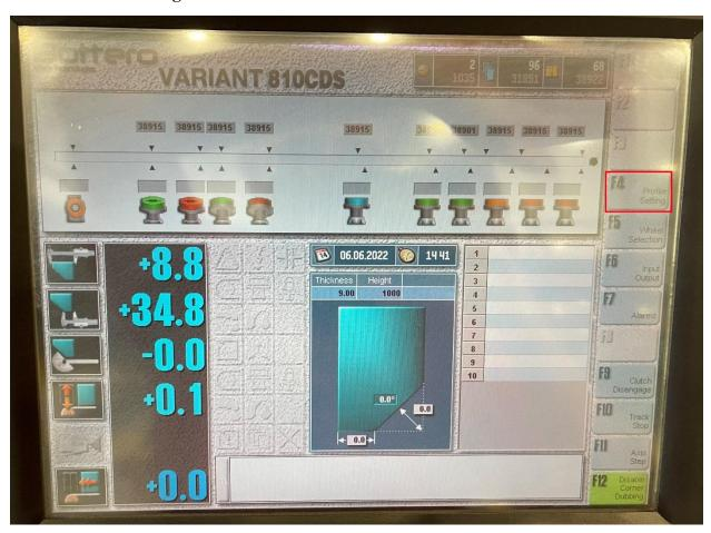
To set the thickness of a glass, select Profile Setting, then enter the thickness of the glass, note that whenever you are going to change the thickness of the glass, you must measure this thickness with a caliper. Note that the thickness of the glass will shows up on the screen with a difference of 2mm,
