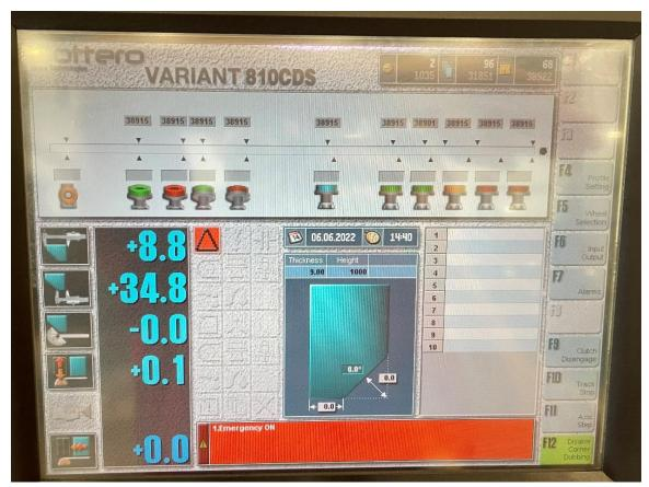
Verify that the dumb corner option is disabled before starting to pass the glass, the light of this option must be turned off, to disable this option, the Disable Corner Dubbling option must be selected.
