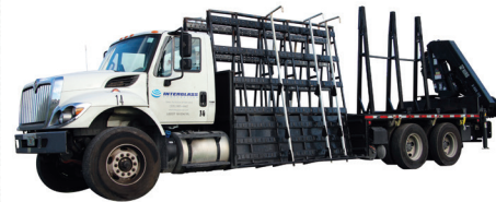
Boom Double-Rack Truck
